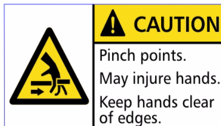
Figure P-2 Pinch Hazard Label: keep Hands Clear
